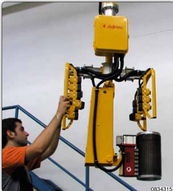
Manipulator equipped with multipolar permanent magnets pneumatically operated, for gripping and lifting steel products.
