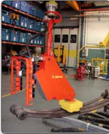
Manipulator equipped with multipolar magnets pneumatically operated for gripping and lifting steel sheets. The distance between centres of the magnets is manually adjustable.
