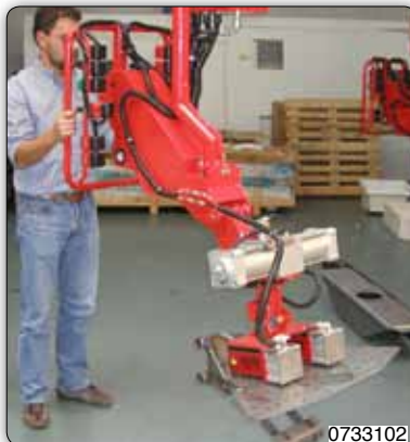
Manipulator with multipolar permanent magnets pneumatically operated, for gripping steel products with inclination up to 90° and rotation up to 180°.
