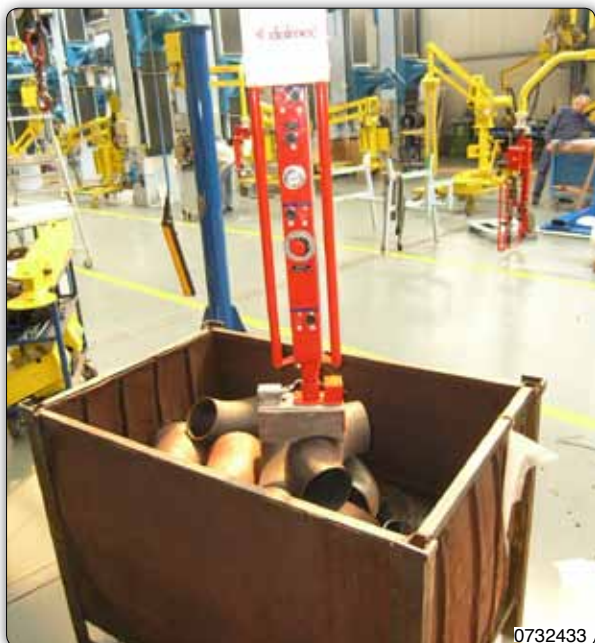
Manipulator with multipolar permanent magnet pneumatically operated, for gripping and lifting steel curves placed jumbled in a container.
