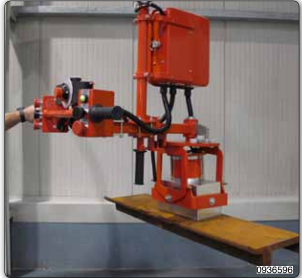
Manipulator equipped with multipolar magnets pneumatically operated for gripping and lifting tracks.
