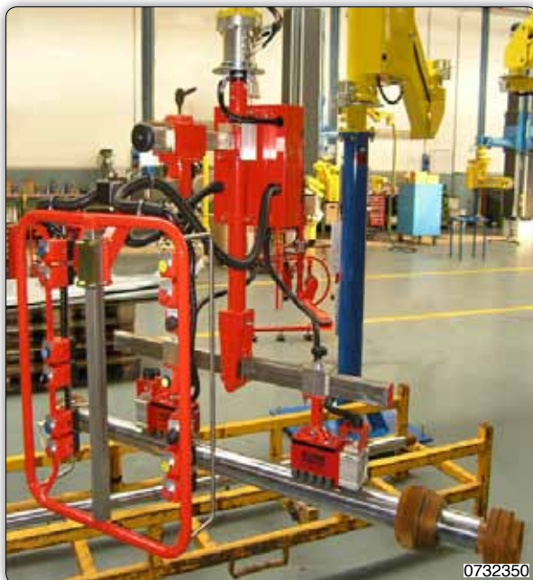
Manipulator equipped with multipolar permanent magnets pneumatically operated, for gripping and lifting steel shafts.
