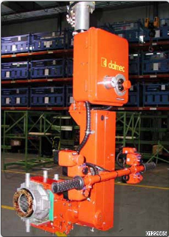
Gripping jaws for handling electric motors on the outside diameter, completed with a pneumatic rotation system.
