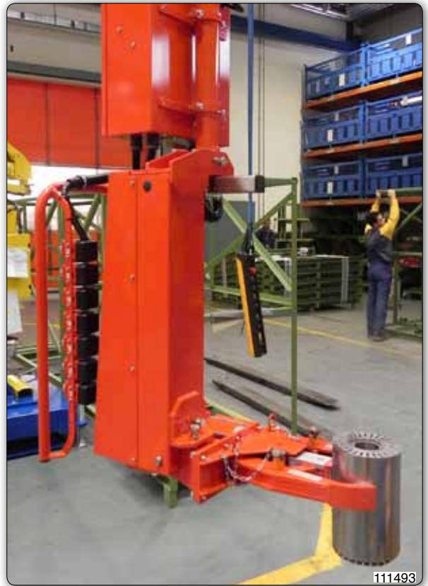
Manipulator equipped with gripping jaws tool for handling rotors on the outside diameter with pneumatic inclination.
