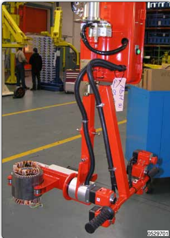
Manipulator equipped with gripping jaws for handling electric stators on the outside diameter, with rotation and manual inclination of the stator.
