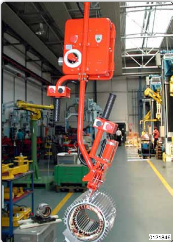
Jaws tooling for gripping and handling electric motors on outside housing.
