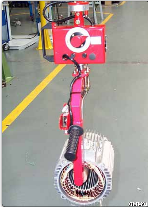
Manipulator equipped with simple round support tooling for handling electric motors.
