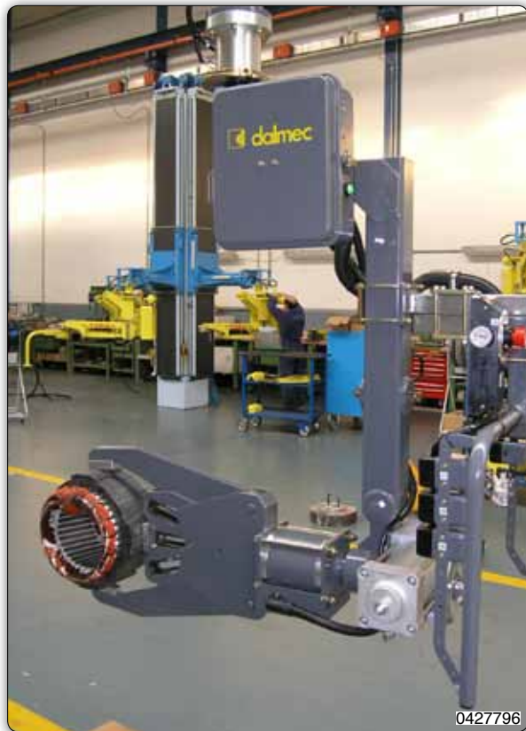
Manipulator equipped with jaws tooling for gripping electric motors on the outside diameter, completed with a pneumatic rotation system.
