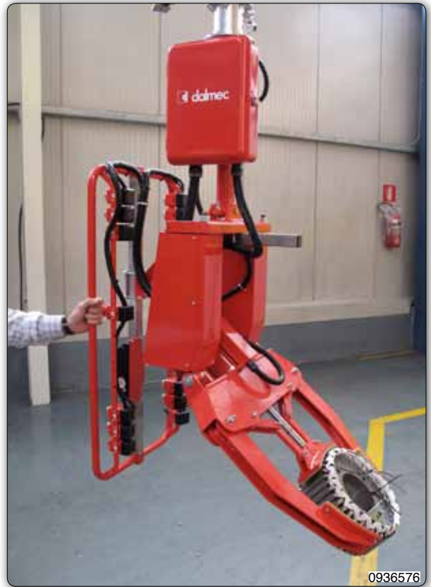
Manipulator equipped with gripping jaws for handling electric stators on the outside diameter, suitable for picking up and handling components from a conveyor and, after a 90° pneumatic rotation, the release on a pallet.
