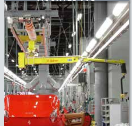
OVERHEAD TROLLEY MOUNTED PFS
